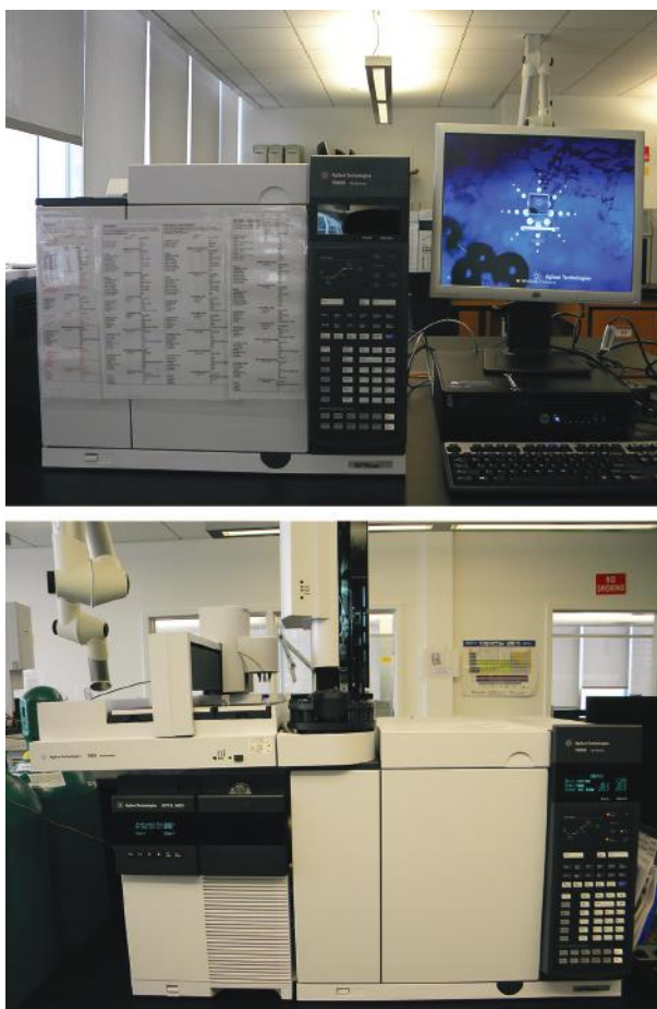
Figure 3.4 Gas chromatograph (top) and gas chromatograph-mass spectrometer (bottom) used for controlled substance analysis. (© Richard C. Li.)
