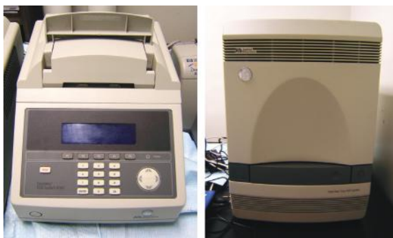
Figure 7.7 Thermal cyclers. A thermal cycler can provide rapid temperature changes as desired to carry out PCR. A PCR thermal cycler (left) and a real-time PCR instrument (right). (© Richard C. Li.)
