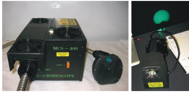
Figure 1.21 Compact alternate light source devices, which are intended specifically for use at crime scenes, reduce search time and improve the recovery of evidence such as biological evidence and chemically enhanced latent fingerprints. (© Richard C. Li.)
