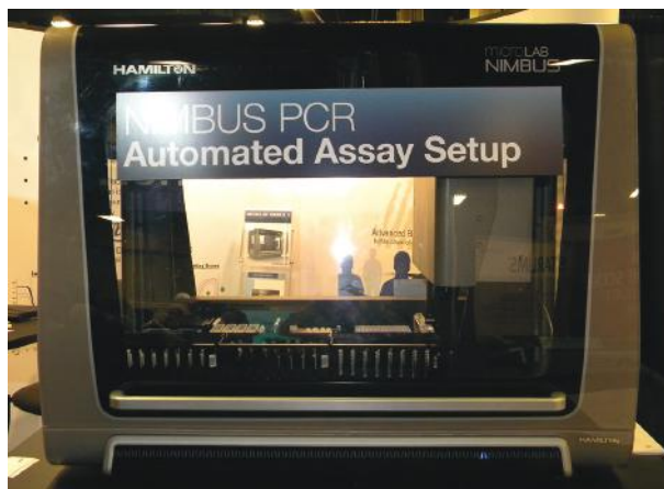
Figure 7.4 A liquid handling workstation for automated PCR assay setup. (© Richard C. Li.)
