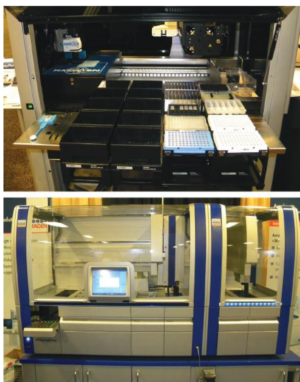
Figure 5.13 Integrated platforms enabling automated DNA sample preparation and liquid handling for subsequent assay setup. These systems utilize silica-coated bead chemistries and can achieve moderate to high throughput of processing (1–96 samples) with bar coding for sample tracking. A Hamilton (top) and a Qiagen system (bottom). (© Richard C. Li.)
