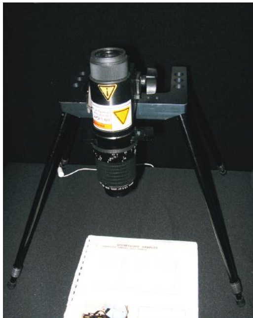
Figure 1.26 A reflected ultraviolet imaging system (RUVIS) imager for documenting close-up views of evidence such as latent fingerprints. (© Richard C. Li.)
