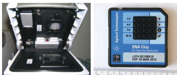
Figure 8.12 A modular instrument for gel electrophoresis. Left: Agilent 2100 Bioanalyzers contain 16-pin electrodes that fit into the wells of a chip. Right: The chip can accommodate sample wells, gel wells, and a well for a size standard. (© Richard C. Li.)
