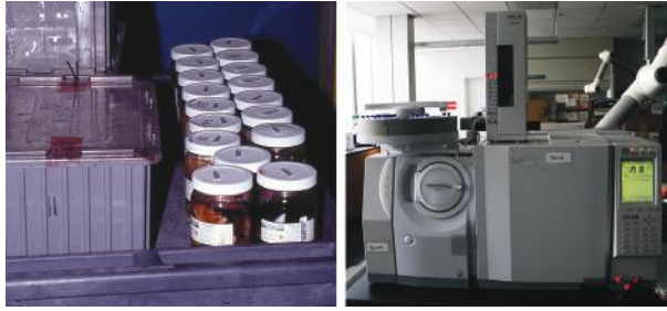
Figure 3.5 Tissue samples (left) and gas chromatograph-mass spectrometer (right) for forensic postmortem toxicological analysis. (© Richard C. Li.)
