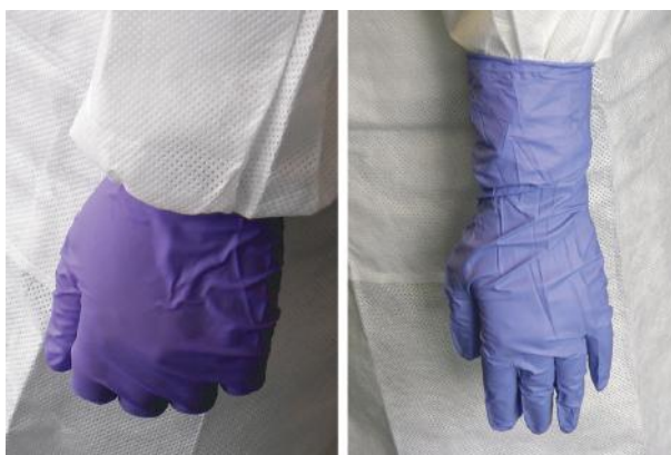
Figure 1.9 Disposable glove (left) and glove with extended cuff (right). (© Richard C. Li.)
