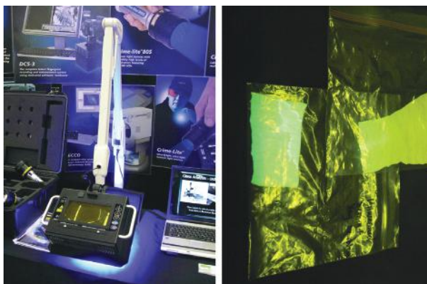
Figure 14.4 A tabletop ALS device (left) for the detection of semen stains (right). (© Richard C. Li.)
