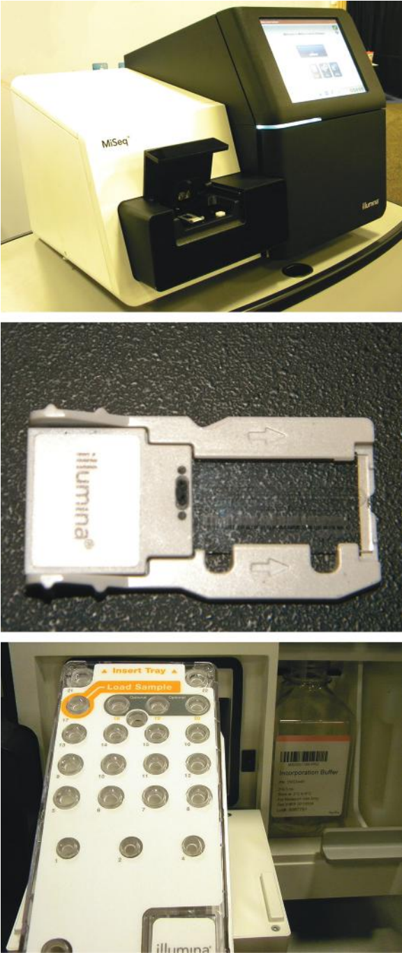
Figure 22.9 A photo of an NGS platform. A MiSeq (Illumina) desktop sequencer (top), a flow-cell device (middle) where DNA templates are distributed for PCR, and a reagent cartridge (bottom) are shown. (© Richard C. Li.)
