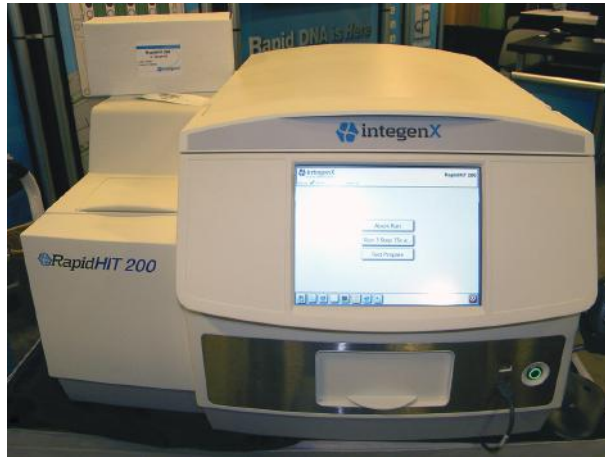
Figure 1.23 An example of a compact Rapid DNA device for processing DNA evidence in the field. (© Richard C. Li.)
