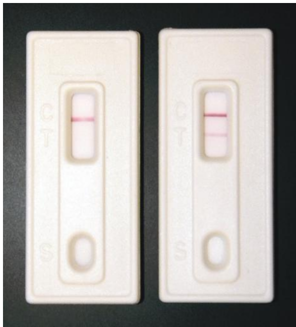
Figure 14.16 Semen identification using an immunochromatographic device (ABAcards PSA). The negative (left) and positive (right) results are shown. The "C" band indicates that the test is valid. The "T" band indicates the presence of human blood. The sample well is labeled as "S". (© Richard C. Li.)
