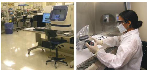
Figure 3.3 A section of a forensic biology laboratory showing an automated electrophoresis instrument used for forensic DNA profiling (left). Processing biological evidence in a biosafety cabinet (right). (© Richard C. Li.)
