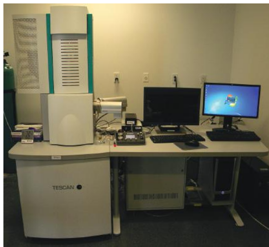
Figure 3.11 Scanning electron microscope used in the analysis of gunshot residue and explosives. (© Richard C. Li.)
