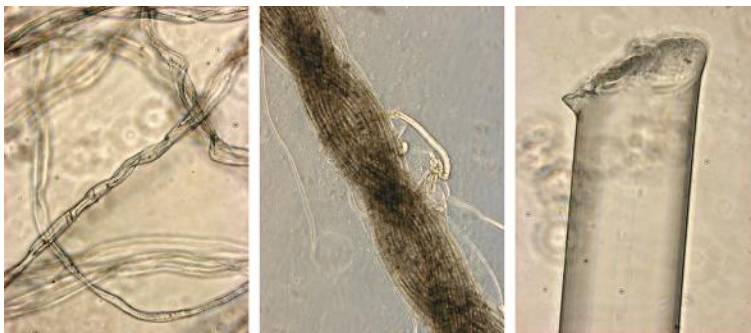
Figure 3.13 Trace evidence: fibers. Cotton (left), nylon (middle), and polyester (right). (© Richard C. Li.)
