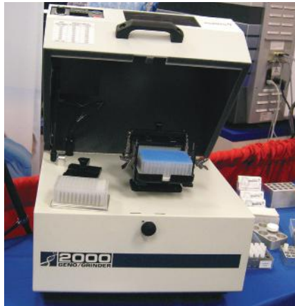
Figure 5.4 An automated mechanical disruption device for efficient disruption of tissues. It can be used for high-throughput applications involving sample preparation for the isolation of nucleic acids. (© Richard C. Li.)
