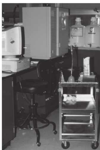
Figure 8.7 Vertical slab polyacrylamide gel. (a) Front and side view of vertical slab polyacrylamide gel apparatus. (b) Automated gel electrophoresis instrument, ABI PRISM 377 ® Genetic Analyzer, which was used in forensic laboratories but is now discontinued. (© Richard C. Li.)
