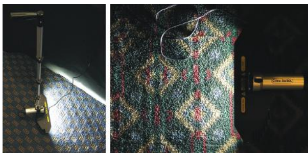
Figure 1.13 A high-intensity light-emitting diode (LED) device for locating evidence at a crime scene is particularly effective in highlighting trace evidence such as hairs, fibers, and shoe prints. (© Richard C. Li.)
