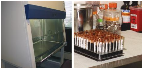
Figure 4.3 Biosafety cabinet for the extraction of DNA from biological evidence (left). Blood samples to be processed in a biosafety cabinet for DNA isolation (right). (© Richard C. Li.)
