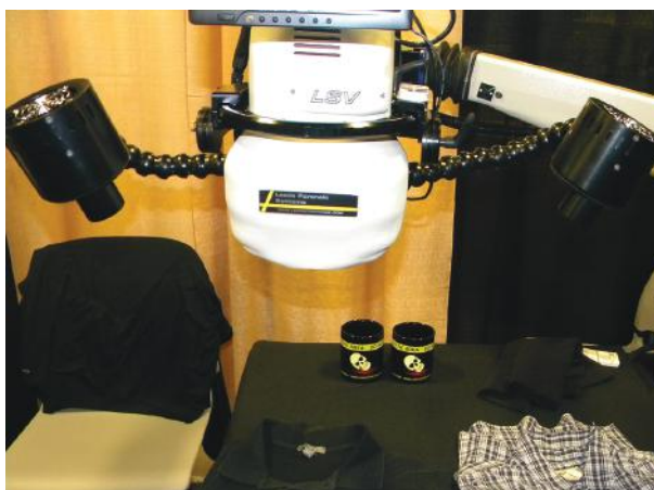
Figure 3.15 A multiwavelength viewing and imaging device used for the examination of various types of evidence, including bodily fluid stains. (© Richard C. Li.)
