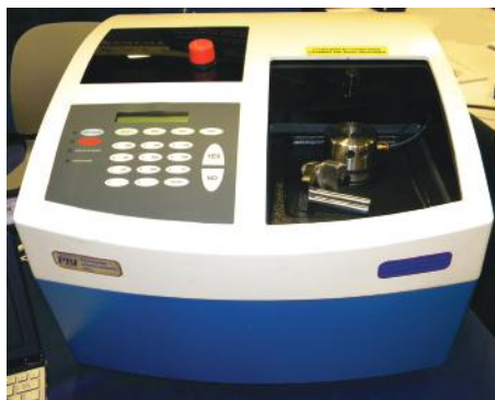
Figure 5.5 Tissue disruption using a pressure-generating instrument also known as a barocycler. During the process, a barocycler is utilized to apply alternating cycles of high and low pressures onto specimens placed in single-use processing containers. The technique is known as pressure-cycling technology (PCT). (© Richard C. Li.)
