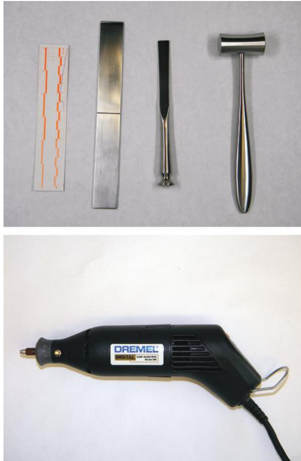
Figure 4.31 Tools for cutting bone samples. Osteotomes and a mallet (top), and a rotary device (bottom). (© Richard C. Li.)
