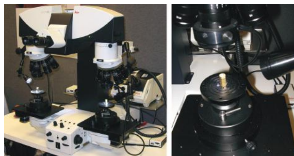
Figure 3.9 A comparison microscope is used for the simultaneous comparison of two items of firearm evidence side by side. (© Richard C. Li.)
