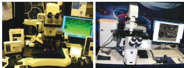
Figure 14.14 A microscopic device for fluorescent detection utilizing SPERM HY-LITER Fluorescent Staining Kit (left) and a laser-capture microdissection device for separating sperm cells from other types of cells (right). (© Richard C. Li.)
