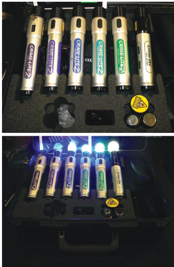
Figure 1.22 LED light sources provide illumination for locating evidence such as bodily fluid stains, hair, or fibers. (© Richard C. Li.)
