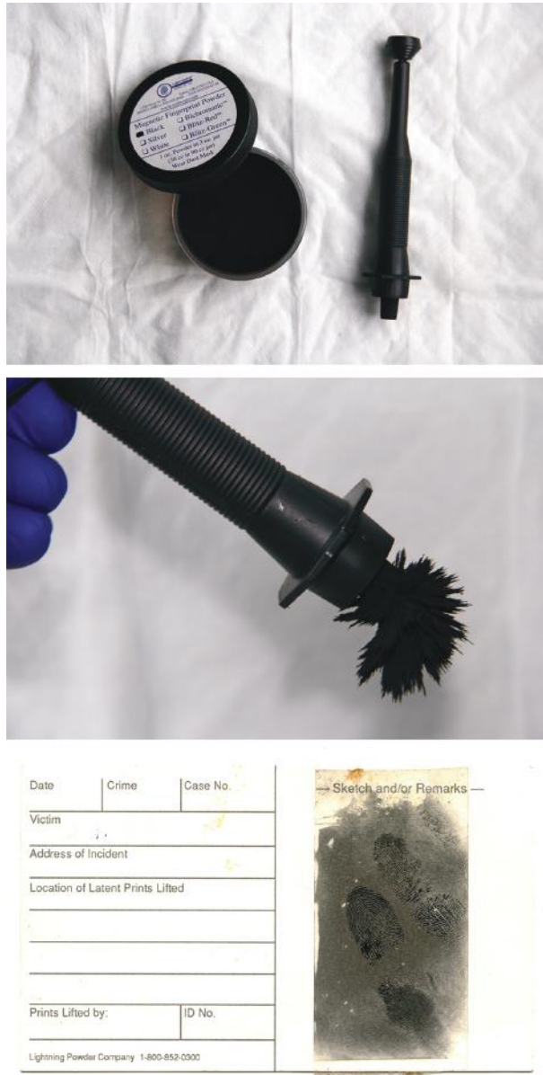
Figure 3.2 Developing latent fingerprints by dusting methods. Using magnetic fingerprint powder (top) that is held by a magnetic applicator (middle). Fingerprints (bottom) dusted by magnetic fingerprint powder, tape lifted and preserved on a fingerprint card. (© Richard C. Li.)
