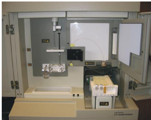
Figure 8.9 A single-capillary electrophoresis instrument, ABI PRISM 310® Genetic Analyzer. This was used in forensic laboratories but is now discontinued. (© Richard C. Li.)
