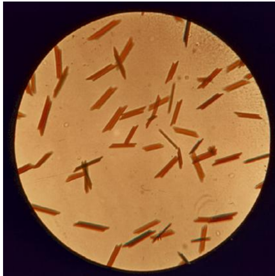
Figure 12.19 Microcrystal assays using the Teichmann method. (From James, S.H., Nordby, J.J., and Bell, S., Forensic Science: An Introduction to Scientific and Investigative Techniques , 4th edn., CRC Press, Boca Raton, 2014. With permission.)
