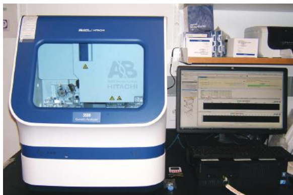
Figure 8.10 Photo of a multicapillary electrophoresis instrument. ABI PRISM 3500® Genetic Analyzer. (© Richard C. Li.)
