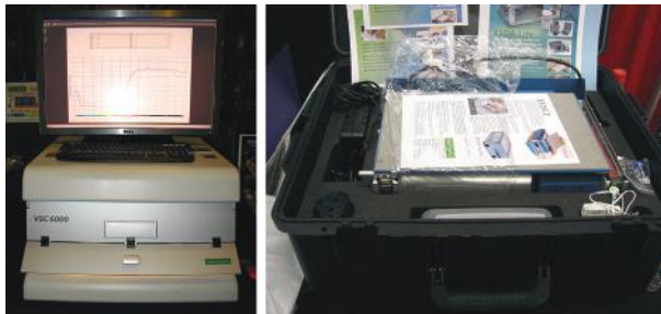
Figure 3.6 A digital imaging system, using multiple illumination sources ranging from ultraviolet to infrared wavelengths, for examining altered and counterfeit documents (left). An electrostatic imaging system for detecting indented writing on questioned documents (right). This device generates an electrostatic image of indented writing, which is then visualized using charge-sensitive toners. (© Richard C. Li.)
