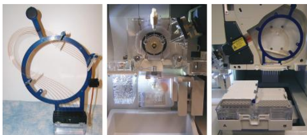
Figure 8.11 Components of the ABI PRISM 3500® Genetic Analyzer. A capillary array (left), electrophoretic buffer chambers (middle), and an autosampler (right). (© Richard C. Li.)
